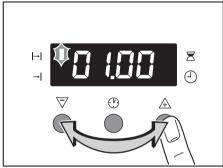
After approx. 5 seconds the display returns to showing the current time. The function indicator Cook time  $|\rightarrow|$  lights up.
